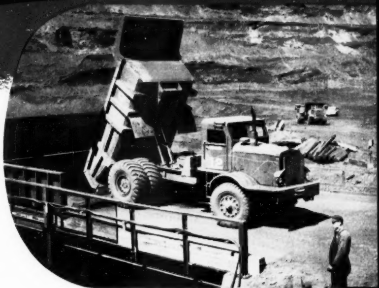
Rear-Dump Euclids—Capacity from 10 to 34 tons—diesel engines from 125 to 400 h.p., spring mounted or semi-rigid drive axles—top speed loaded up to 35.7 m.p.h.
